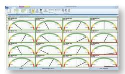
**MeasurLink Process Manager** displays snapshot windows of characteristics that are currently being collected in MeasurLink Real-Time. The data can be sorted by station, capability or time stamp.
