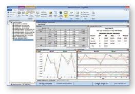
In addition to the standard calculations, the software provides graphical tools for analysis of the measurement system. The Xbar and R chart can show whether there is adequate gage discrimination to record part to part variation in production and if operators are consistent. The Part-by-Appraiser plot can show if there is a lack of consistency between operator inspection techniques.
