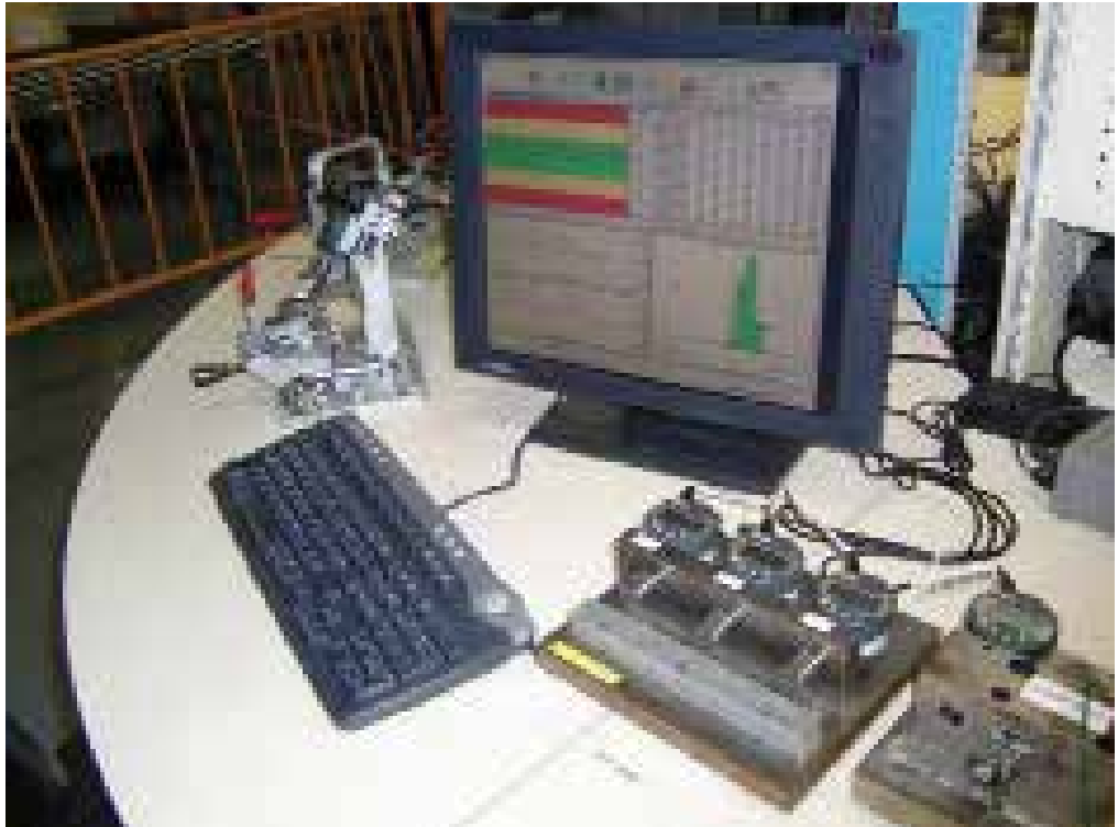
Electricfil QA work station for measuring Hall sensor dimensions. Station employs fixtures with integrated digital gages connected to a Mitutoyo MeasurLink measurement data management system.
